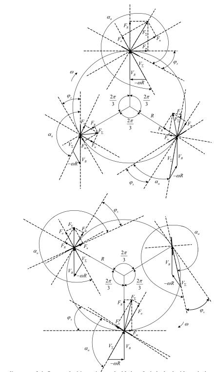
Fig 1. Vector diagrams of air fluxes velocities acting on the blades of wind wheel with vertical rotation axis and forces, created by these fluxes at non – zero values of blade turn angle, constructed for two, shifted by 180°, positions of wind wheel.
