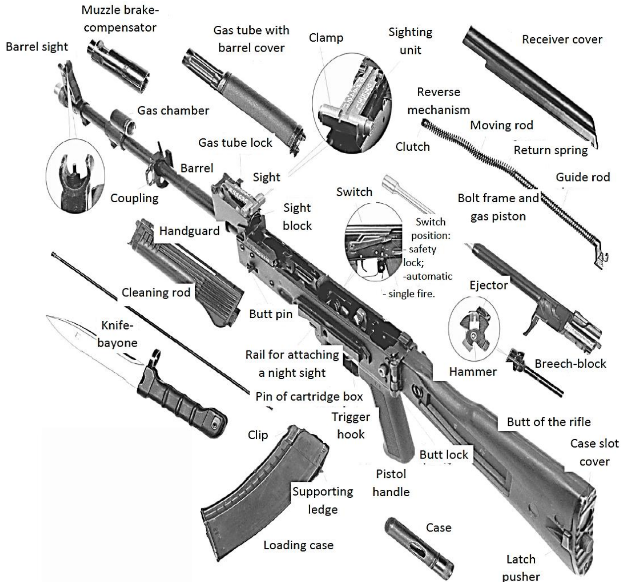
Fig. 3. Main components and mechanisms of AK-74M assault rifle [13]
