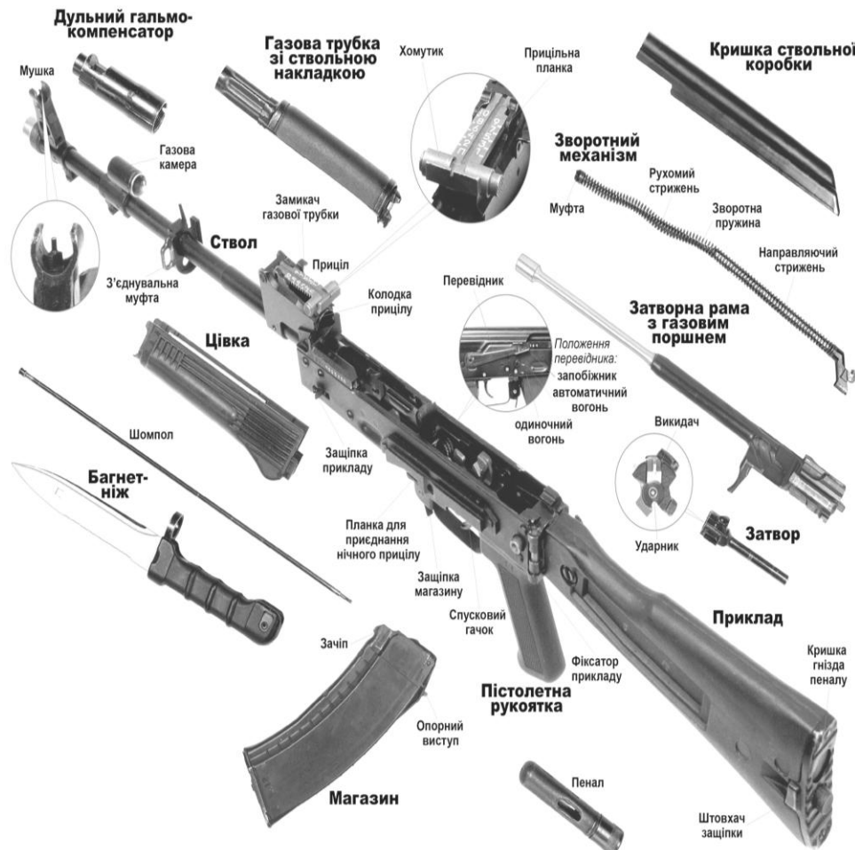
Fig. 3. Main components and mechanisms of AK-74M assault rifle [13]
