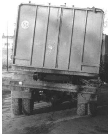
Fig. 4. Roll of the dustcart in the direction of the manipulator in case of the side loading of SMW in the body of the dustcart
