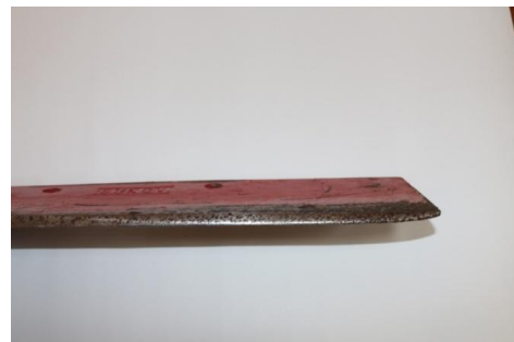
Fig. 12. Results of the atmospheric corrosion on the friction surfaces of tillage machines working tools during off season storage after the operation
