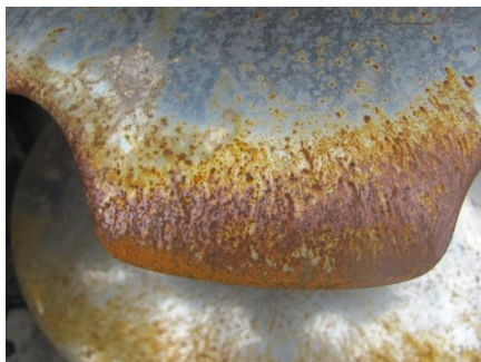
Fig. 12. Results of the atmospheric corrosion on the friction surfaces of tillage machines working tools during off season storage after the operation
