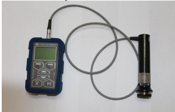
Fig. 8. Micro durometer T-YД2, used for the determination of the microhardness of the friction surfaces of the tillage machines working tools
