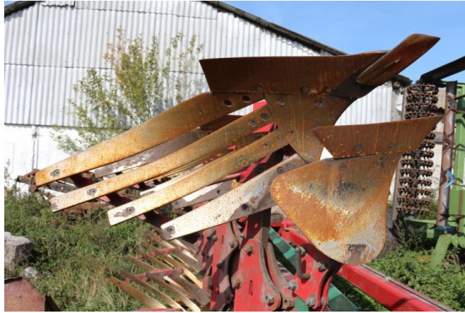
Fig. 7. Photo of the friction surface of the tillage machine working tool in the period of the off season storage
