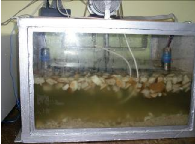
Fig. 3. Environment stratification of a reactor without vibroactivation
