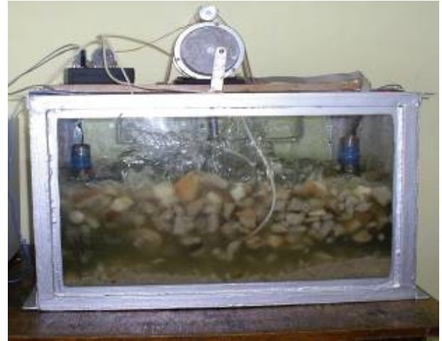
Fig 4. Vibrating intensification of heat exchange transfer in a reactor
