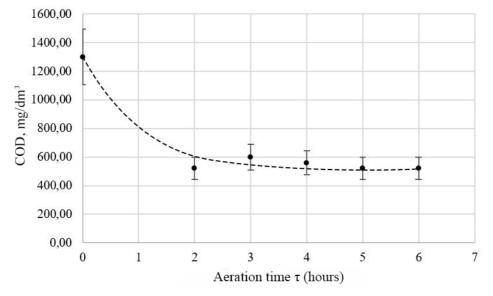
Fig. 1. Kinetics of the waste water treatment process at paper mill according to COD index
