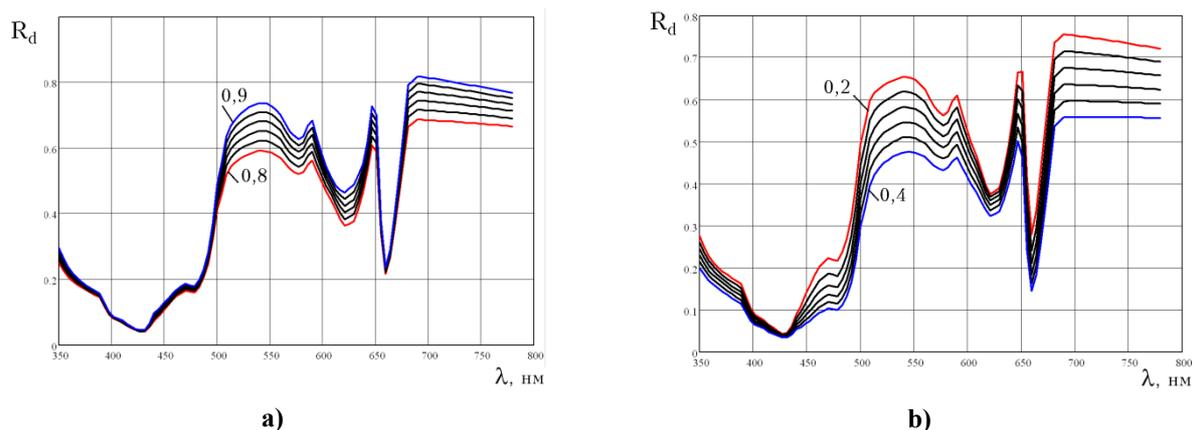
Fig. 1. Spectral characteristics of the diffuse reflection factor on the surface of the aquatic habitat on the change of the phytoplankton pigment parameters: a) relation between the chlorophyll *a* and general chlorophyll from 0.8 to 0.9; b) relation between the carotenoids and general chlorophyll from 0.2 to 0.4
