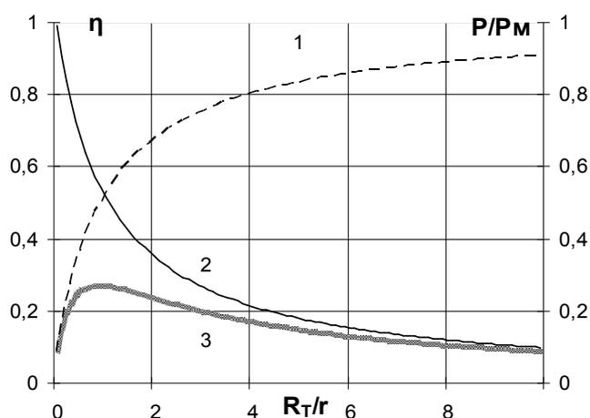
Fig. 1. Efficiency factor (1) and the character of the full (2) and useful (3) powers change (in relative coordinates calculated for certain values of e. m. f. and  $r$ ) in the circuit of the electric heater, depending on the parameter  $\frac{R_T}{r}$ .
