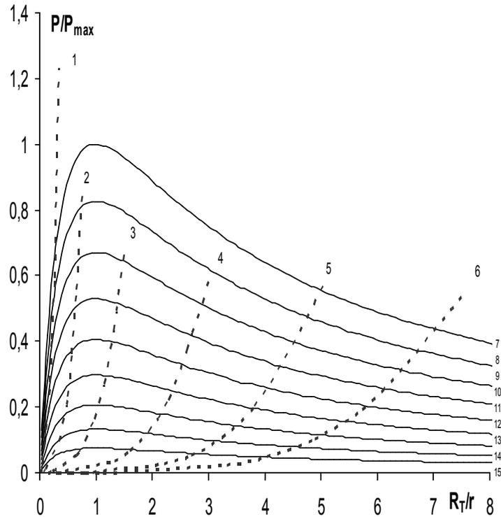
Fig. 2. Dependences of the heating lines 7 – 15 and dissipated by the similar in form band electric heaters of different electric resistance of lines 1 – 6 of  $P$  powers (rated for maximum), on the relation  $\frac{R_T}{r}$
