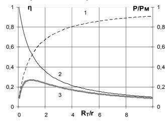
Fig. 1. Efficiency factor (1) and the character of the full (2) and useful (3) powers change (in relative coordinates calculated for certain values of e. m. f. and r) in the circuit of the electric heater, depending on the parameter  $\frac{R_T}{r}$ .
