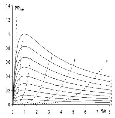
Fig. 2. Dependences of the heating lines 7 – 15 and dissipated by the siminar in form band electric heaters of different electric resistance of lines 1 – 6 of P powers (rated for maximum), on the relation  $\frac{R_T}{r}$
