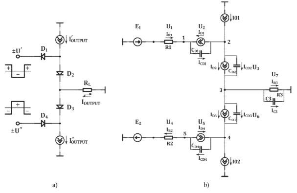
Fig. 2. The circuit of commutation unit at the diode switches: a) general view; b) equivalent circuit Taking into account, that [13]
