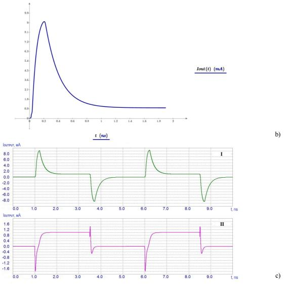
Fig. 3. Transient processes during the diode switch commutation, graphs: a) the switch closure process; b) the switch opening process; c) on the results of simulation in Microcap software (I – for high-frequency diode; II – for the transistor in the diode connection)
