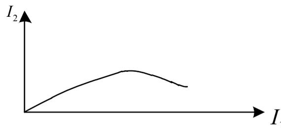
Fig. 1. Indicative graph of the real output static characteristic  $I_2 = f(I_1)$  of the instrument current transformer
