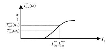
Fig. 4. Dependence graph  $T_{opt}^* = f_4(I_{1m}) = f_4(\sqrt{2}I_1) = f_5(I_1)$
