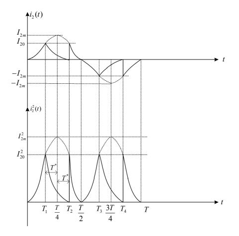
Fig. 2. Graph of the current  $i_2(t)$  and its square  $(i_2(t))^2$  during the period T
