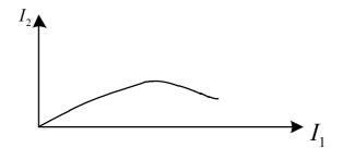
Fig. 1. Indicative graph of the real output static characteristic  $I_2 = f(I_1)$  of the instrument current transformer
