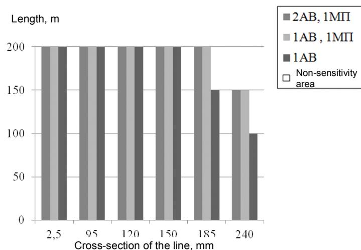
Fig. 6. Area of switching devices resistance account in the equivalent resistance of shop-floor grid with 10 radial lines
