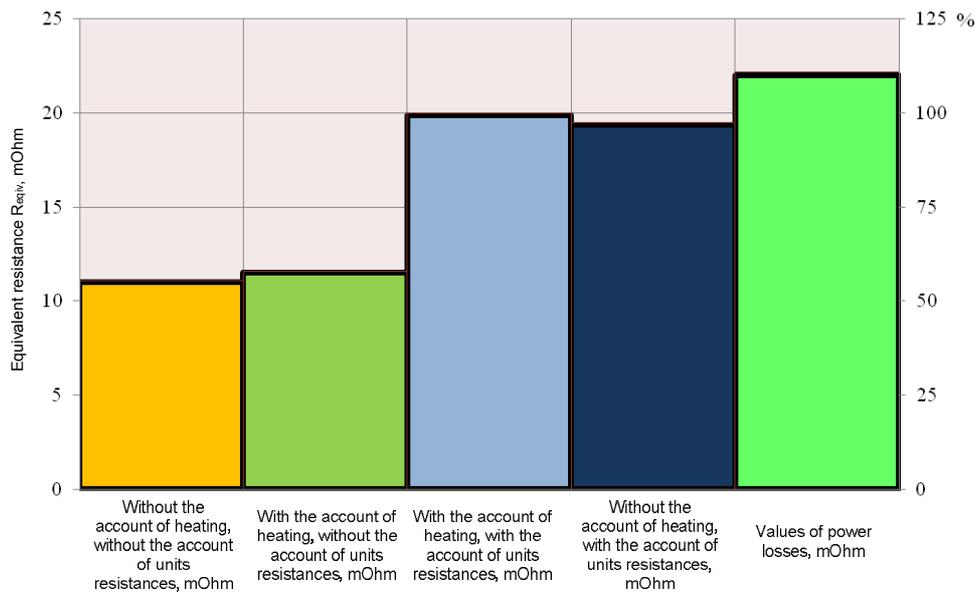
Fig. 2. Value of the equivalent resistance of shop-floor section of the grid with the account of the impact of main parameters of the equipment
