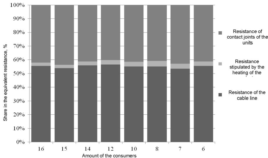
Fig. 3. Ratio in the equivalent resistance of the radial grid the resistance of the contact joints of low voltage units and the resistance of the lines, with the account of conductors heating
