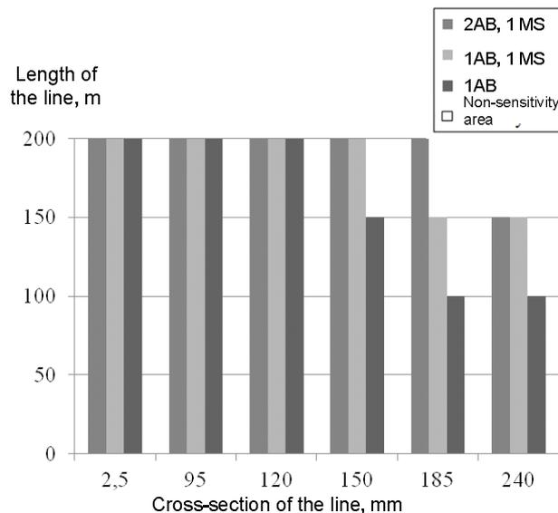
Fig. 5. Area of the account of switching devices resistance in the equivalent resistance of shop-floor grid with 6 radial lines
