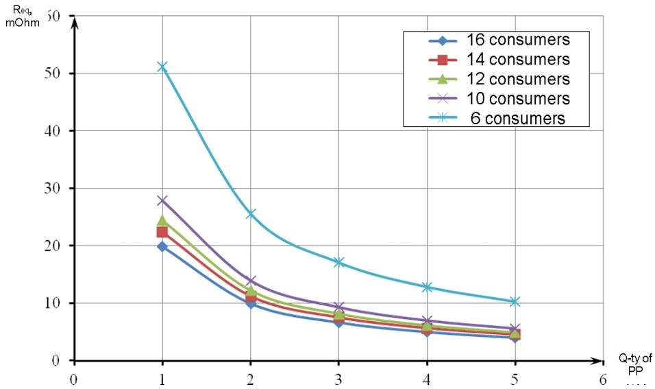
Fig. 4. Dependence of the equivalent resistance of the grid on the number of power points connected in parallel
