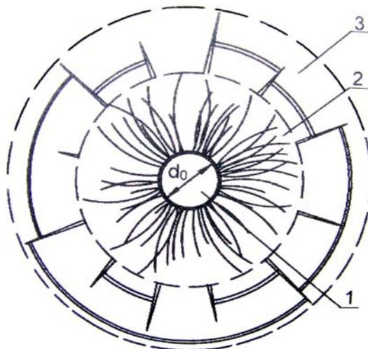
Fig. 3. The Schematic image of an integrated picture of defects in isolator after its pulse breakdown
