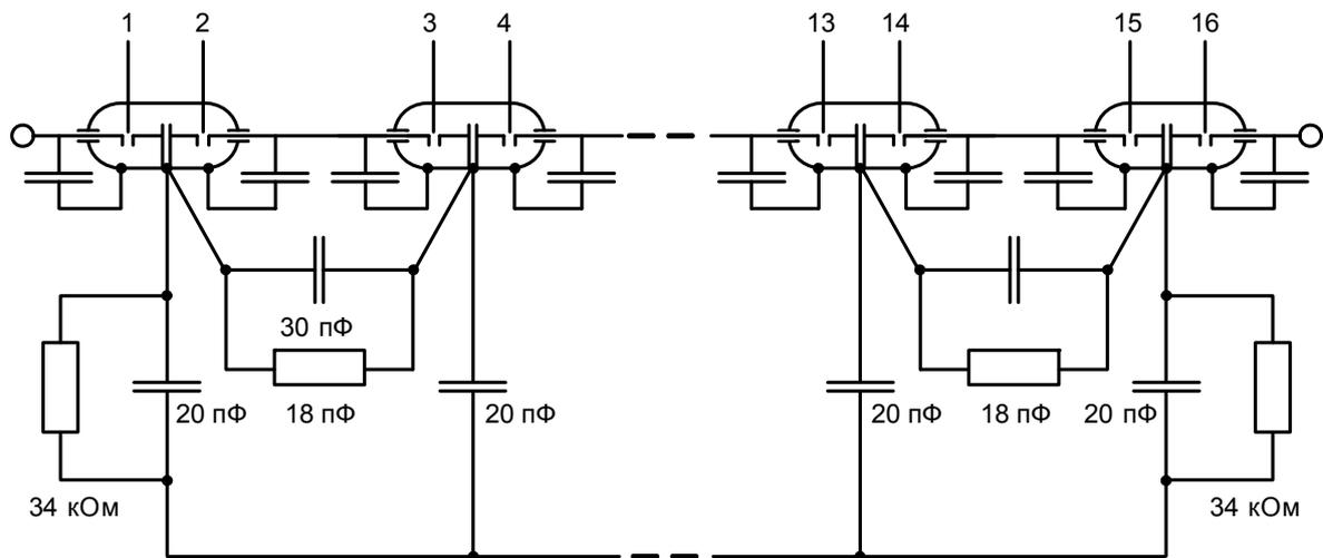
Fig. 1. Electrical schematic diagram of switch VVB-750 kV
