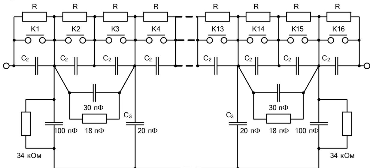
Fig. 2. The equivalent circuit of the switch for incoming impulse voltage of a lightning origin
