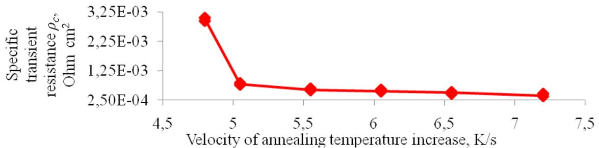
Fig.4. Dependence of specific transient resistance of ohmic contacts  $\rho_c$  on the velocity of annealing temperature increase.
