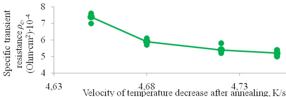
Fig. 5. Dependence of specific transient resistance of ohmic contacts  $\rho_c$  on the velocity of contact cooling
