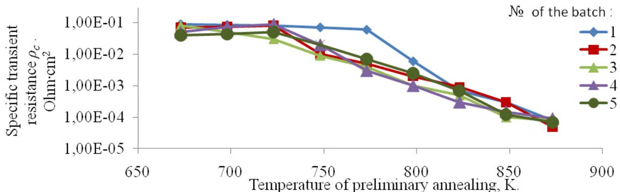
Fig. 1. Impact of preliminary annealing of the substrate on specific transient resistance of the contact  $Ag-Ge-In/n-n^+GaAs$
