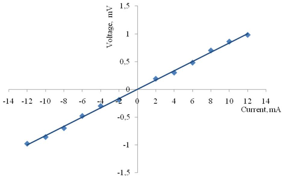
Fig. 3. Voltage-current characteristic of ohmic contact *Ag-Ge-In/n-n<sup>+</sup>GaAs*
