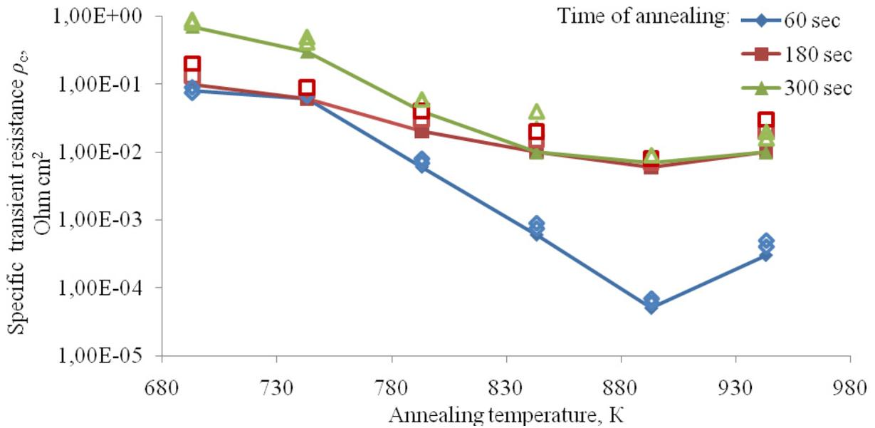
Fig. 2. Impact of the temperature and time of annealing on specific transient resistance  $\rho_c$  of *Ag-Ge-In/n-n<sup>+</sup>GaAs* contacts
