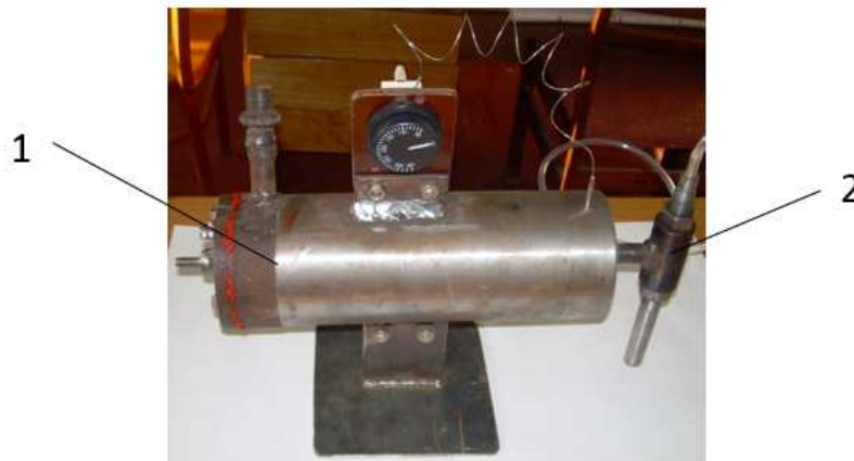
Fig. 1. The unit for gas dynamic spraying of functional coatings: 1 – air heater, 2 – powder sprayer
