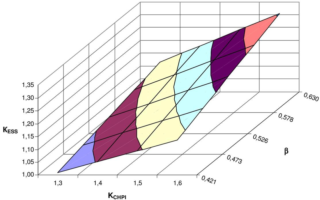
Fig. 1. Area of high energy efficiency of ESS with CHPI of small power for heat supply, on conditions of minimal efficiency of GPE and peak fuel-fired boiler
