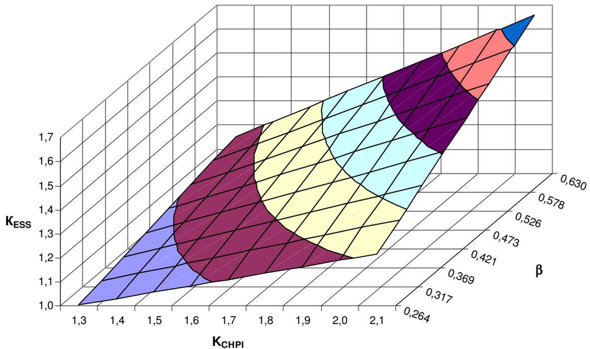
Fig. 2. Area of high energy efficiency of ESS with CHPI of small power for heat supply, on conditions of maximum efficiency of GPE and peak fuel-fired boiler
