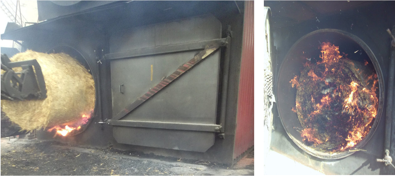
Fig. 2. The process of straw bale loading in thermal generator and burning
