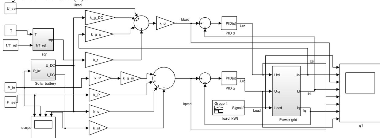
Fig. 2. Computer-based model for verification of operation adequacy of regulators d and q of current components of the inverter
