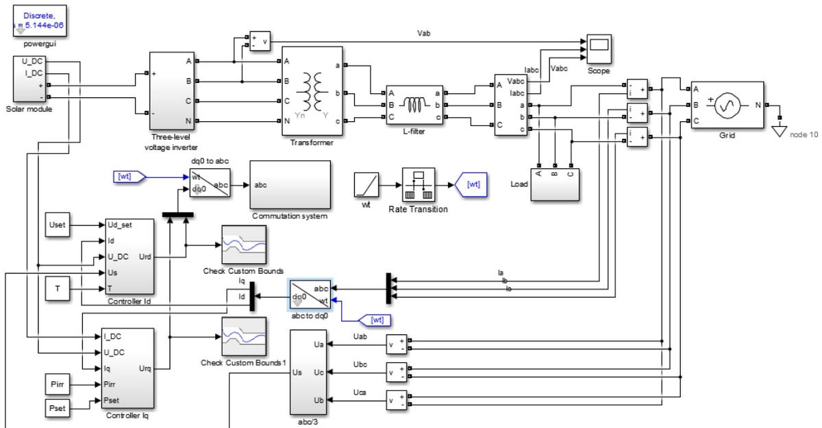
Fig. 5. Computer-based model, that corresponds to circuit hardware components of multilevel current inverter
