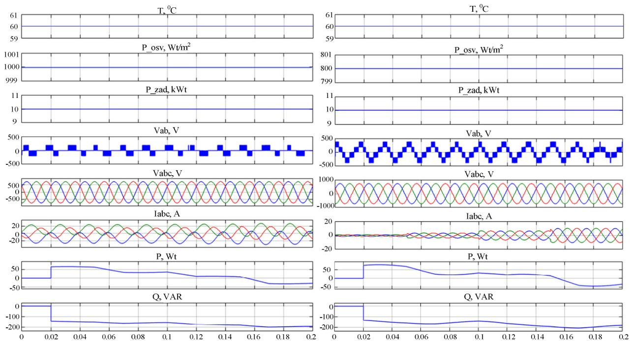
Fig. 7. Graphs of transient processes of the control system of multilevel voltage inverter at various settings of regulators
