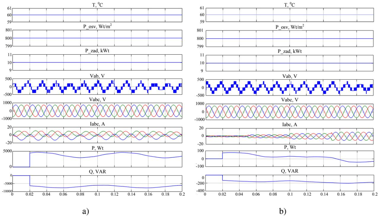
Fig. 8. Graphs of transient processes of the control system of multilevel networking voltage inverter with non-compensated filter (a) and filter with automatic compensation (b)
