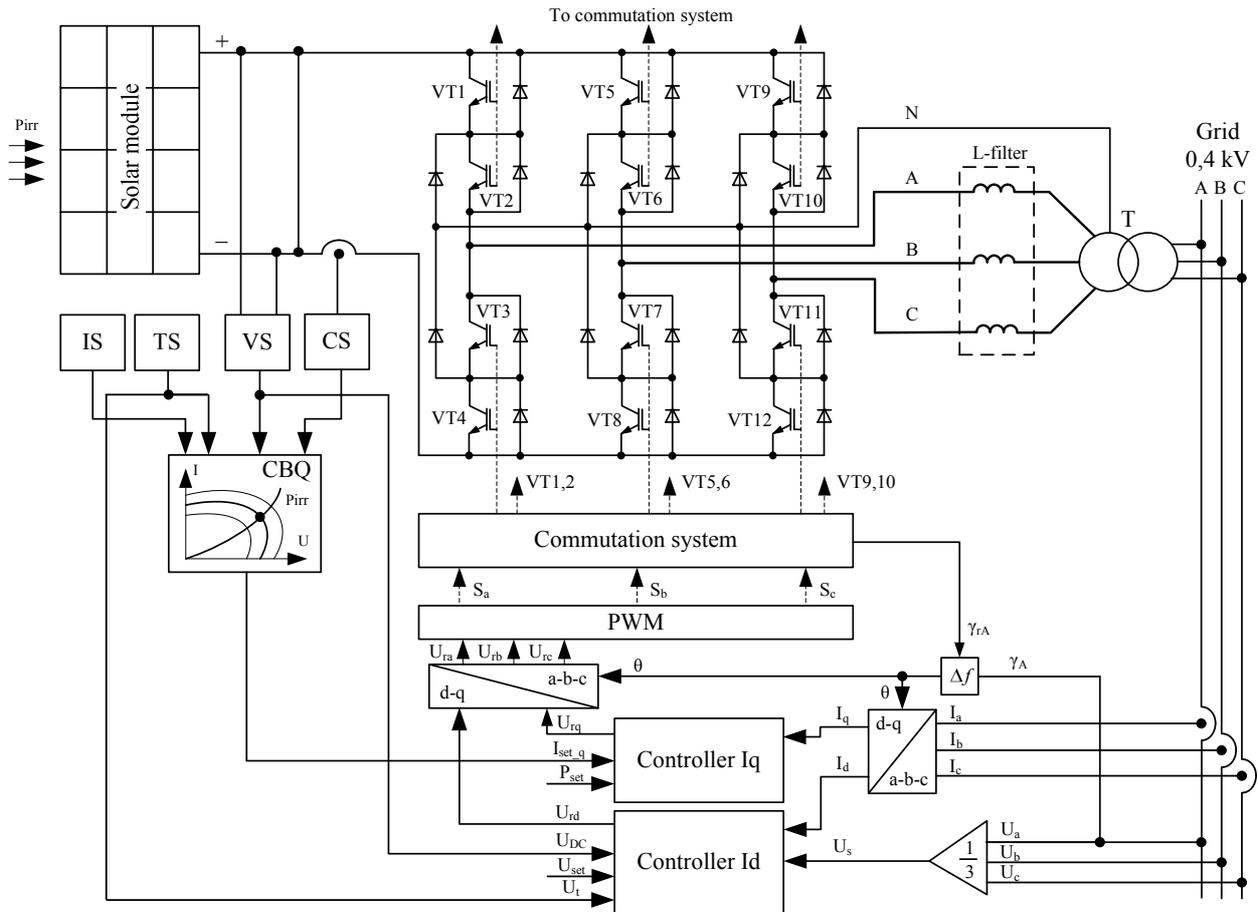
Fig. 1. Functional diagram of three-level networking inverter with internal circuits for regulation of the currents  $I_d$  and  $I_q$
