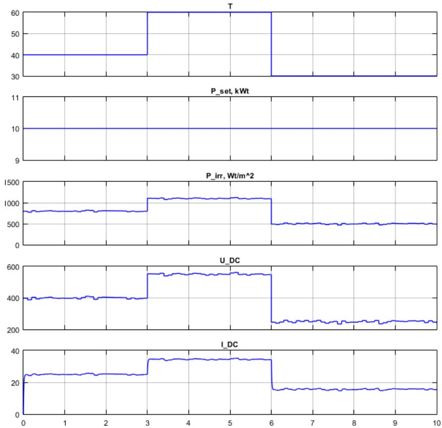
Fig. 4. Specified and realvalues of lightning level, output current and solar cell voltage
