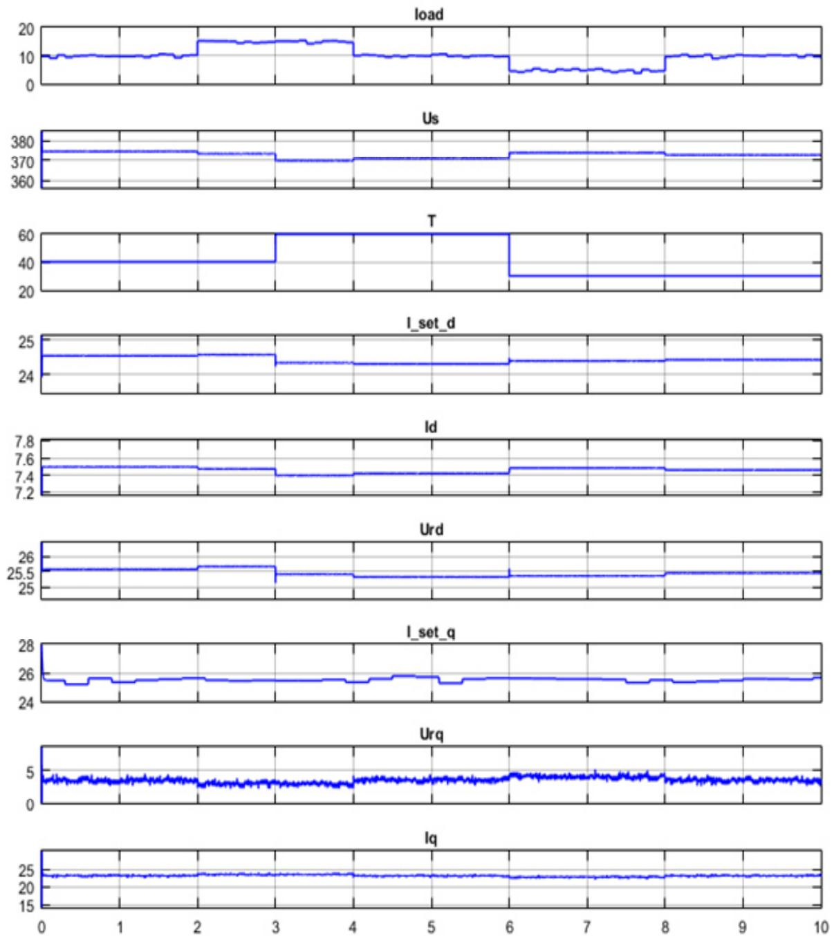
Fig. 3. Simulation results for PID-regulators of longitudinal and transversal components of inverter current
