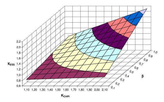
Fig. 6. Values of dimensionless criterion of ESS for energy efficiency operation modes of CHPI, on conditions of minimal efficiency of peak hot-water fuel-fired boiler
