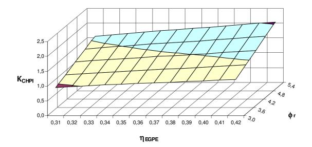
Fig. 1. Area of energy efficient operation of small power CHPI by dimensionless criterion of CHPI energy efficiency, depending on real values of HPI coefficient of performance and efficient factor of GPE Наукові праці ВНТУ, 2016, № 1
