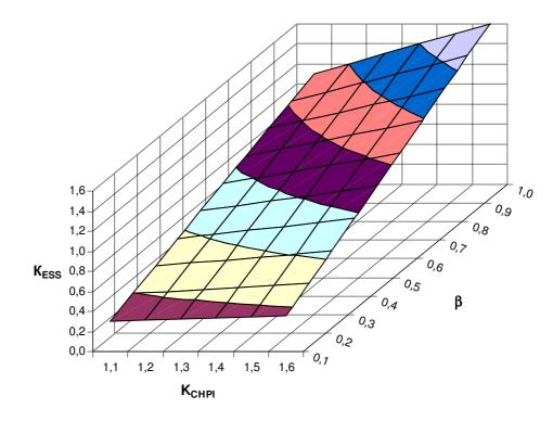
Fig. 4. Values of dimensionless criterion of energy efficiency of small power ESS, on condition of minimal efficiency of GPE and PSH, with the consumption of electric energy by peak electric boiler from CHPI
