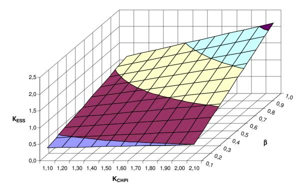
Fig. 5. Values of dimensionless criterion of energy efficiency of small power ESS, on condition of maximum efficiency of GPE and PSH, with the consumption of electric energy by peak electric boiler from CHPI
