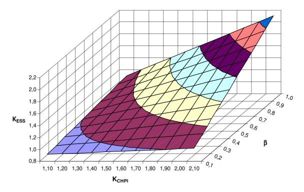
Fig. 7. Values of dimensionless criterion of ESS for energy efficiency operation modes of CHPI, on conditions of maximum efficiency of peak hot-water fuel-fired boiler
