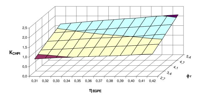
Fig. 2. Area of energy efficient operation of large power CHPI by dimensionless criterion of CHPI energy efficiency, depending on real values of HPI coefficient of performance and efficient factor of GPE
