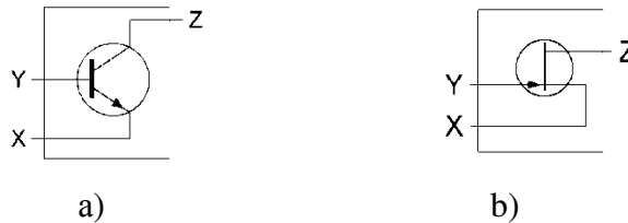
Fig. 2. Single – transistor current conveyors CCII - on bipolar (a) and field effect (b) transistors
