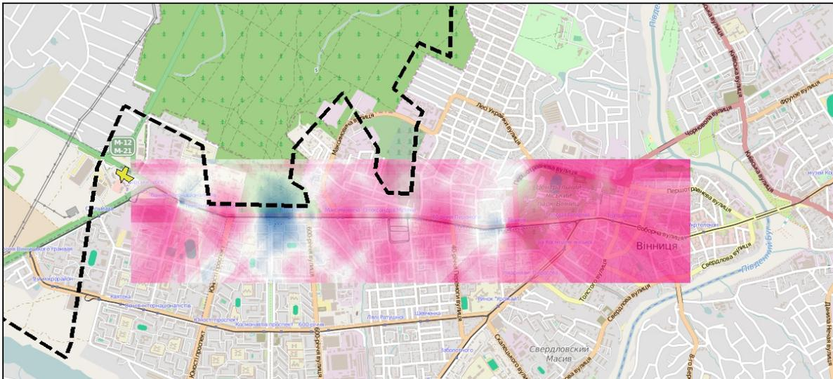
Fig. 4. Interpolation of the second route monitoring data by the method of cricking
