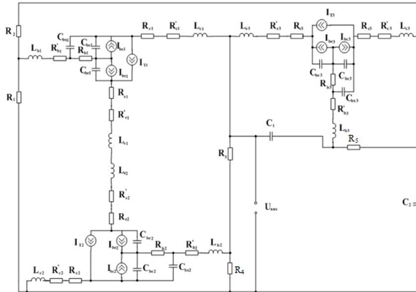
Fig. 2. Equivalent circuit of the converter on the basis of two bipolar transistors with active inductive element
