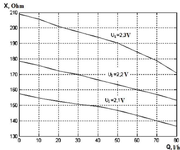
Fig. 4. Theoretical dependence of reactive component of output impedance on expenses
