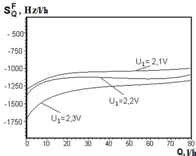
Fig. 7. Dependence of sensitivity on gas consumption
