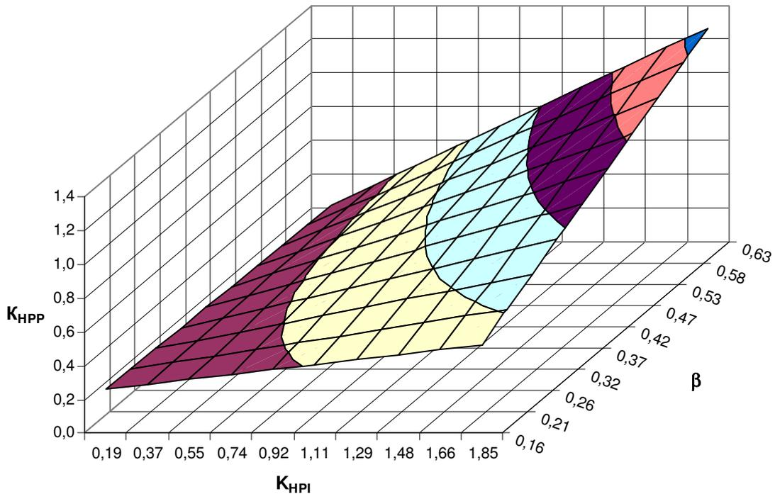
Fig. 9 – Values of dimensionless criterion of energy efficiency of small capacity HPP with electric drive for optimal values of HPI load share, on condition of electric energy consumption from GTI
