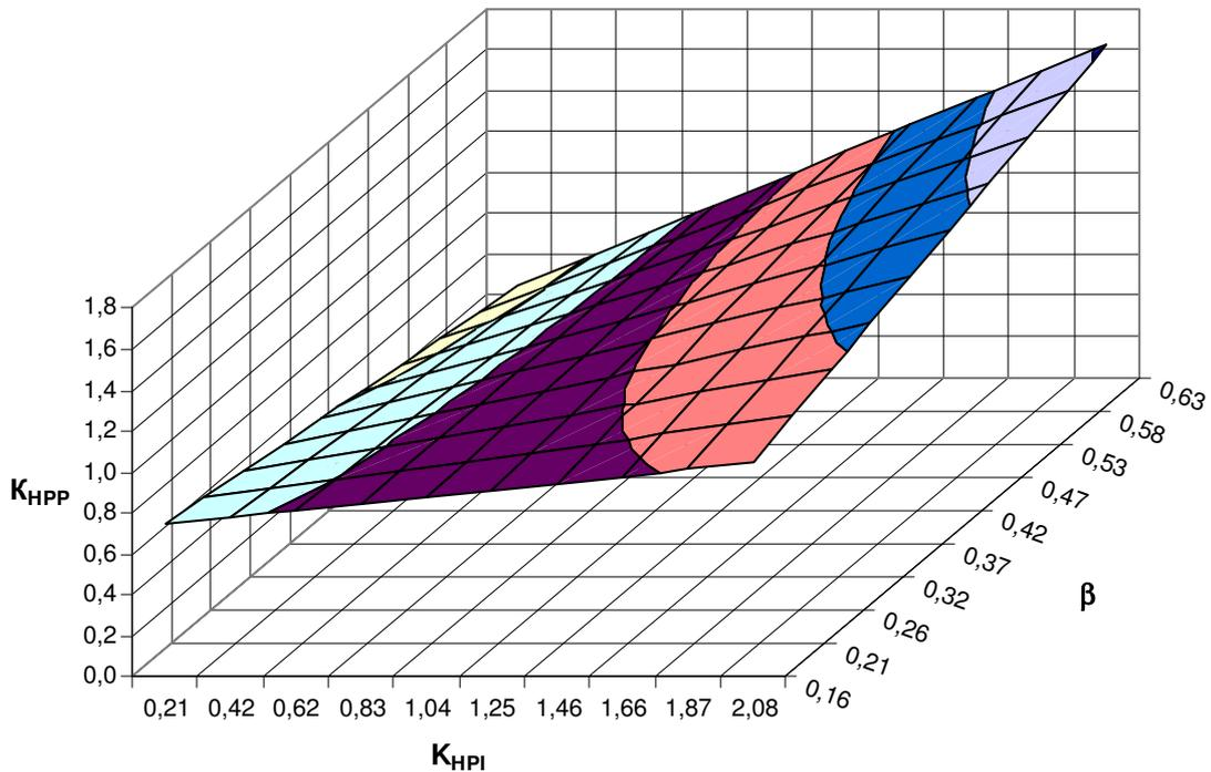
Fig. 12 – Values of dimensionless criterion of energy efficiency of large capacity HPP with electric drive for optimal values of HPI load share, on condition of electric energy consumption from GTI
