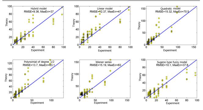
Fig. 4. Verification of the models on the test set
