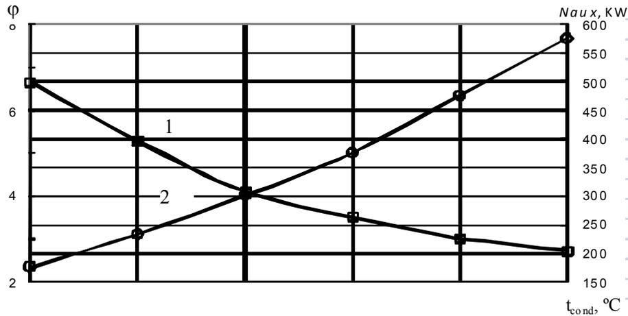
Fig. 3. Current values of the heating factor  $\varphi$  (line 1) and electric power of the auxiliaries –  $N_{aux}$  (line 2)
