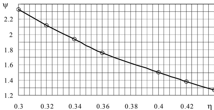
Fig. 2. Dependence of  $\Psi$  on the efficiency of steam turbine plants
