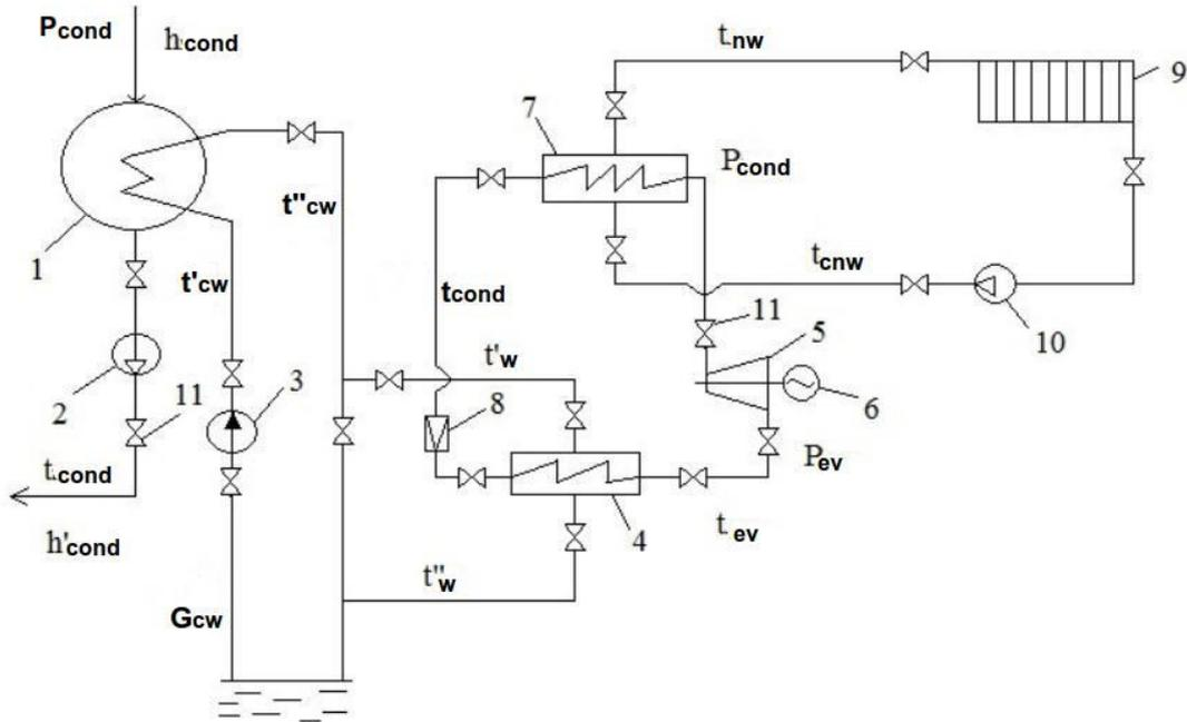
Fig. 1. Diagram of heat pumping station, powered from the condenser of steam turbine: 1 – condenser of steam turbine; 2 – condensate pump; 3 – circulating pump; 4 – HPS evaporator; 5 – compressor; 6 – electric drive of HPS compressor; 7 – HPS condenser; 8 – throttle valve; 9 – heat load; 10 – networking pump; 11 – shut off valve
