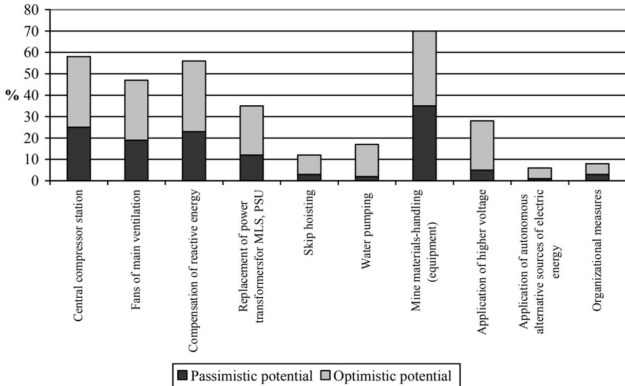
Fig. 2. Comparison of optimistic and pessimistic potentials of energy efficiency increase of the elements of the systems of energy supply and electric equipment of iron-ore mines
