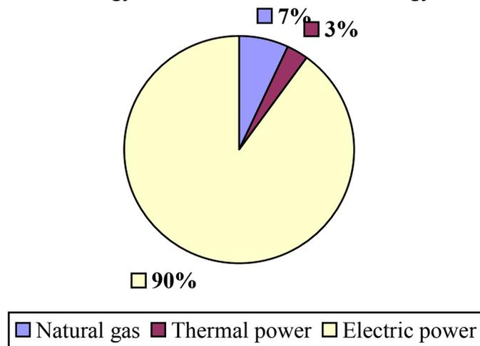
Fig. 1. Diagram of power costs components at iron-ore enterprises with underground method of ore mining
