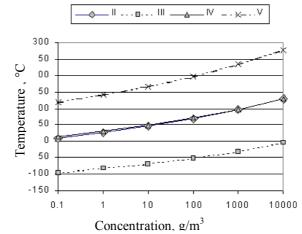
Fig. 2. Dependence of tar dew point temperature on its concentration
