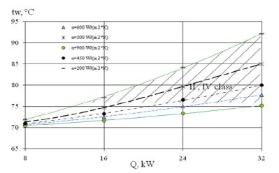
Fig. 3. Dependence of boiler heat exchanger wall temperature on the side of gases on the load (water cooling)
