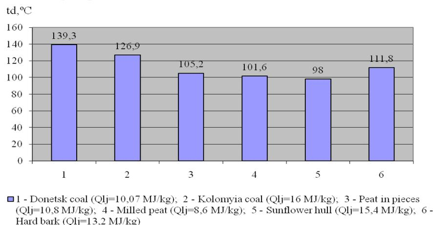
Fig 1 Dependence of dew point temperature on the kind of low-grade fuel
