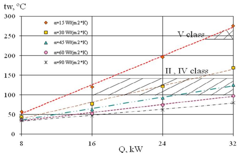
Fig. 4. Dependence of boiler heat exchanger wall temperature on the side of gases on the load
