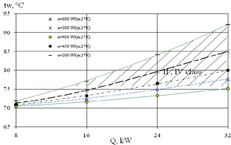
Fig. 3. Dependence of boiler heat exchanger wall temperature on the side of gases on the load (water cooling)
