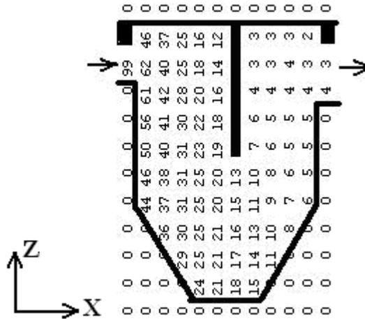
Fig. 2. The pollutant concentration distribution in the vertical settler with a partition (side view, cross-section  $y=2,25$ m,  $w_s=1,2$ m / h,  $C_{\max}=100$ )
