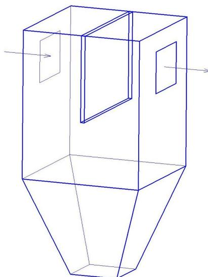
Fig. 1. Scheme of the vertical settler with a partition
