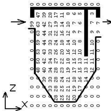
Fig. 6. The pollutant concentration distribution in a vertical settler with a partition shifted to the outlet (side view, cross-section  $y = 2,25$  m,  $w_s = 1,2$  m / h,  $C_{\max} = 100$ ).
