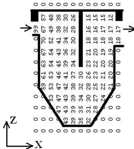
Fig. 3. The pollutant concentration distribution in the vertical settler with a partition (side view, cross-section  $y=2,25$  m,  $w_s=0,5$  m / h,  $C_{\max}=100$ )
