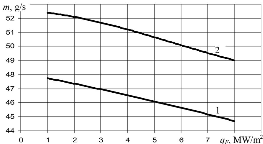
Fig. 5. Influence of  $q_F$  on the mass emission  $SO_2$  under condition  $\alpha_F=1,2$  and  $\Delta\alpha=0,2,1$  – heating oil; 2– coal
