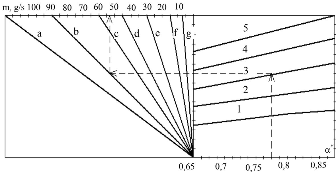
Fig. 3. Nomographic chart for the determination of specific mass emission of sulfur oxide in to the atmosphere: 1 –  $V_G=4 \text{ m}^3/\text{kg}$ ; 2 – 6; 3 – 8; 4 – 10; 5 – 12; a –  $A=4$ ; b – 3; c – 2; d – 1,5; e – 1; f – 0,5; g – 0,2
