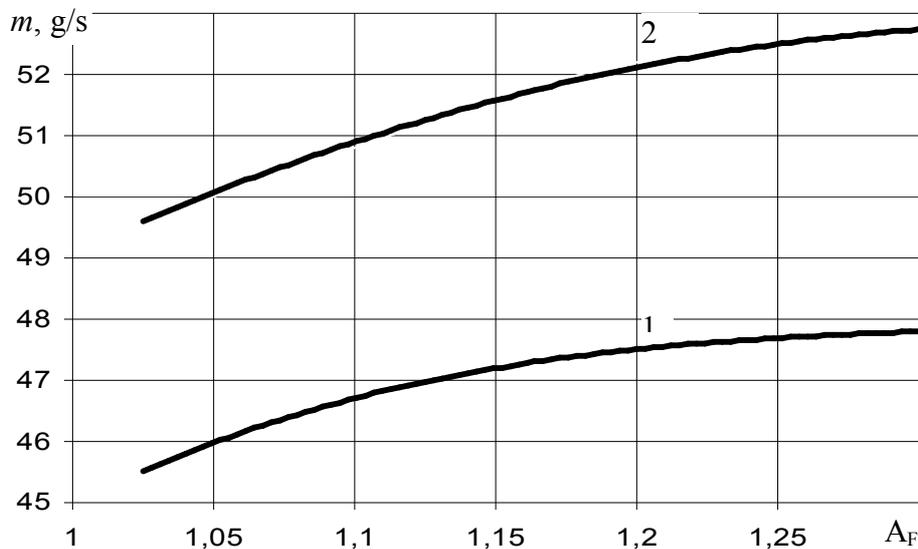
Fig. 4. Current values of mass emissions of sulfur oxide under condition that  $q_F=2$  MJ/m<sup>2</sup>, and air inflow ratio equals  $\Delta\alpha=0,2$ ; 1 – heating oil; 2 – coal
