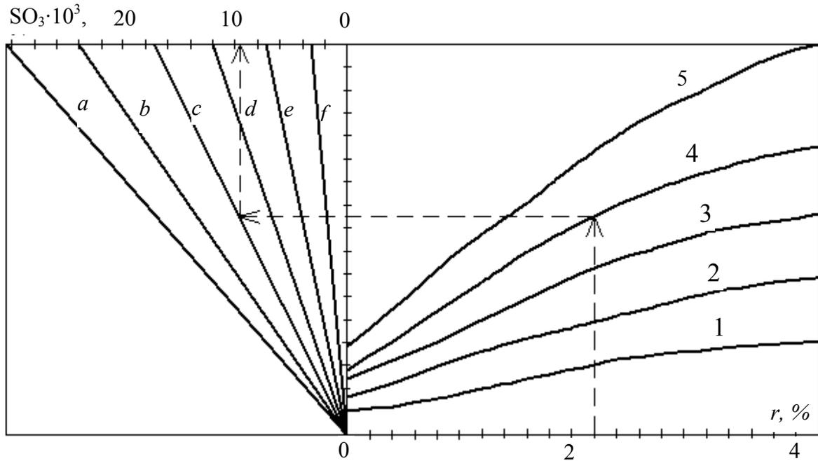
Fig. 2. Nomogram for determination of  $\text{SO}_3$  percentage in combustion products : 1 –  $\beta=0,5 \cdot 10^{-3}$ ; 2 – 1; 3 – 2; 4 – 0,5; 5 – 4; a –  $q_F=9 \text{ MW/m}^2$ ; b – 7; c – 5; d – 3; e – 2; f – 1
