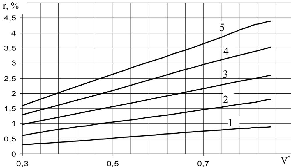
Fig. 1. Content of excessive air in combustion products: 1 –  $\alpha_T=1,05$ ; 2 – 1,1; 3 – 1,15; 4 – 1,2; 5 – 1,25
