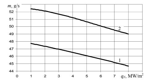
Fig. 5. Influence of  $q_F$  on the mass emission SO<sub>2</sub> under condition  $\alpha_F = 1,2$  and  $\Delta \alpha = 0,2,1$  – heating oil; 2– coal
