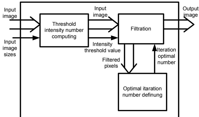
Fig. 2. The functional scheme of the adaptive filter of speckle noise on the US image
