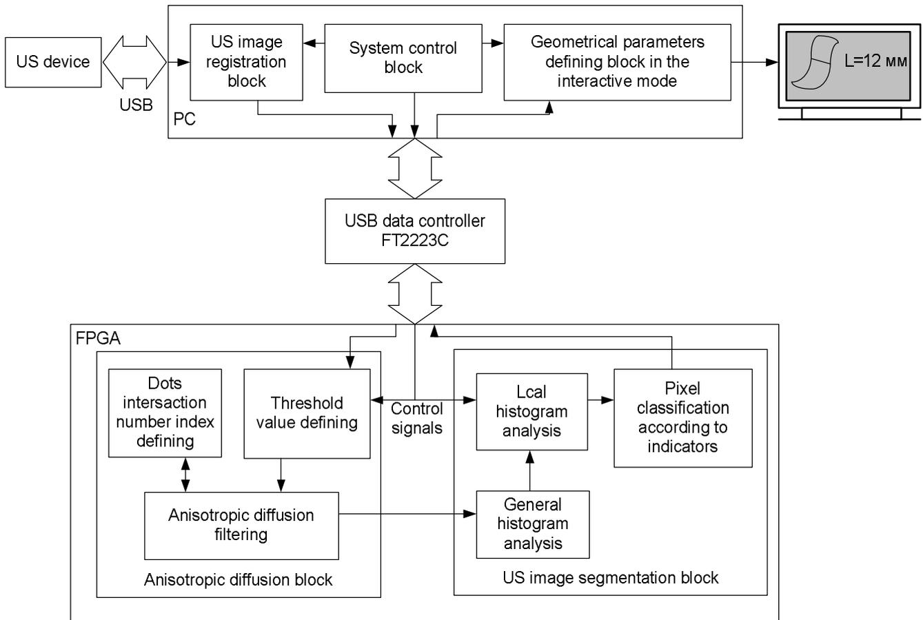
Fig. 1. Structural and functional diagram of the hard-and software device for the evaluation of geometrical parameters of gall bladder on US images
