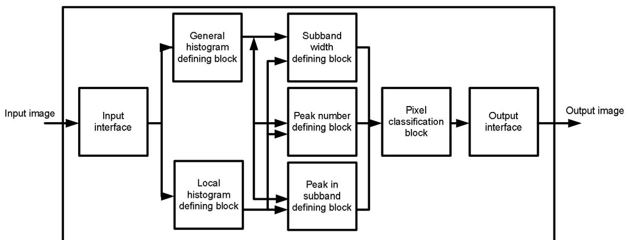
Fig. 3. The functional scheme of the US image segmentator
