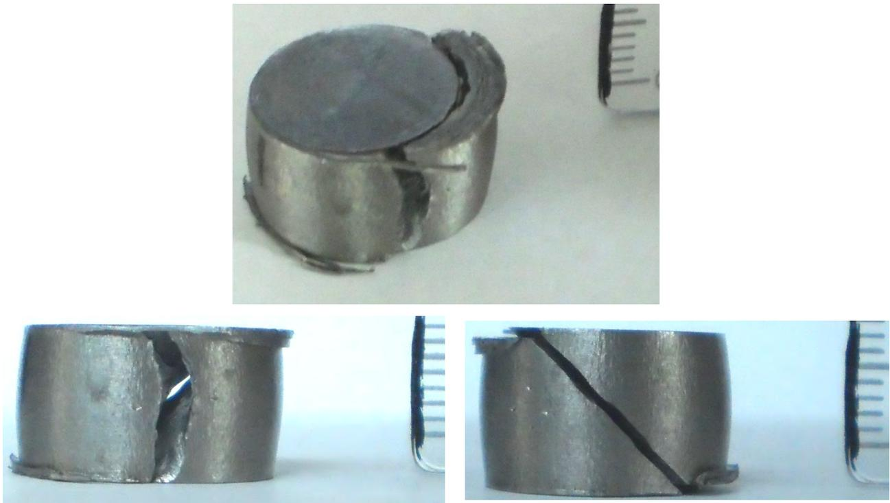
Fig. 7. Rupture of the specimen, mode of alloy BT9 while axisymmetric setting
