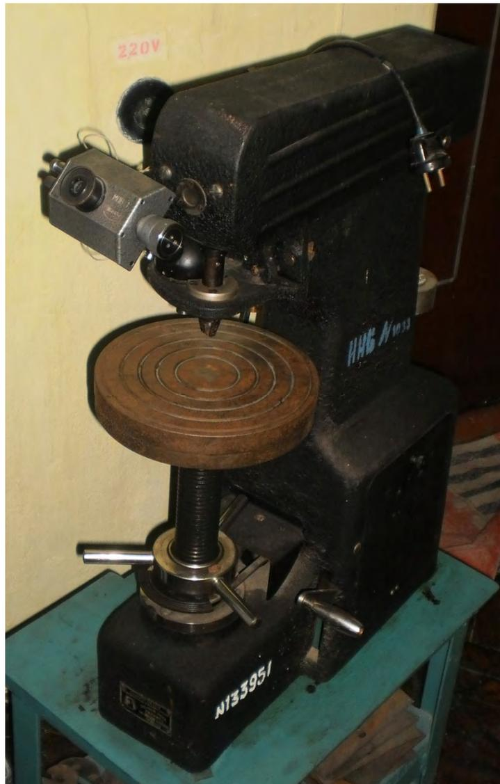
Fig. 1. Vickers hardness tester of TII type
