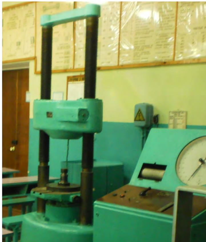
Fig. 5. General view of hydraulic press ПИММ-125
