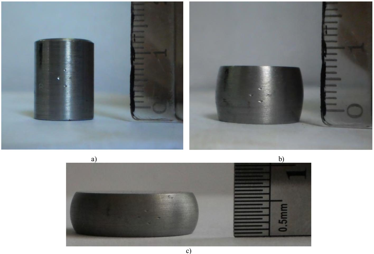
Fig. 8. Cylindrical specimen, mode of steel 45: a) before axisymmetric setting; b) after loading 20 t.; c) after loading 31,5 t.
