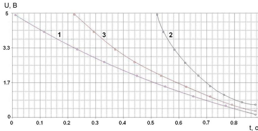
Fig. 4. Output sensor characteristics: 1 – in the first channel exponentiator; 2 – in the second channel exponentiator; 3 – in the output of the system
