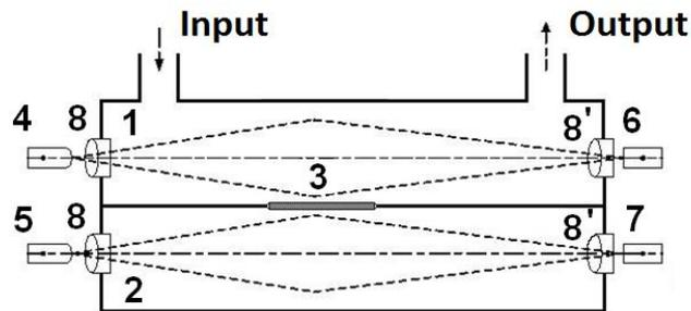
Fig. 2. The diagram of the optic gas concentration sensor :
