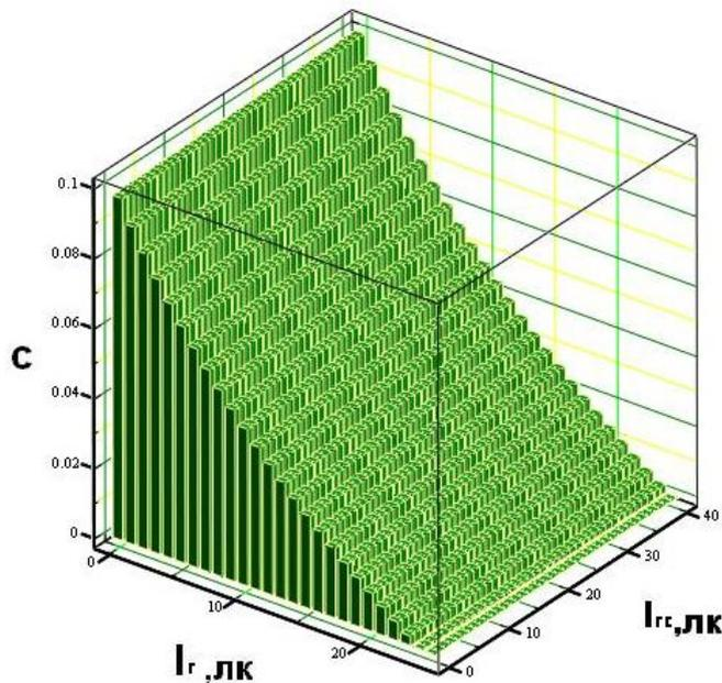
Fig. 1. The graph of dependence of gas impurities concentration on emission intensity
