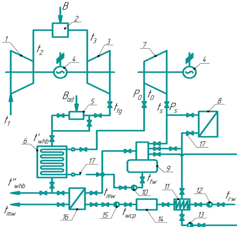
Fig. 1. Basic thermal block diagram of gas steam unit:
