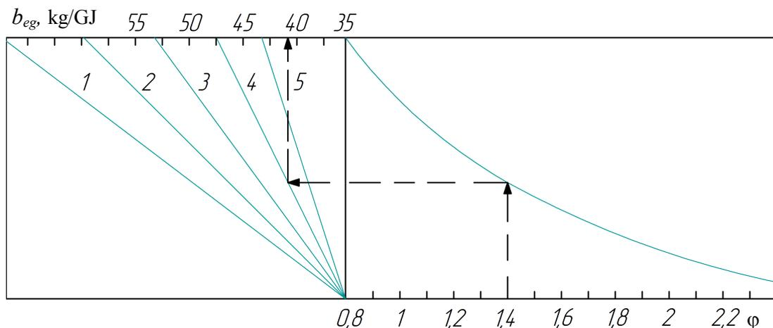
Fig. 4. Nomograph for determination of specific consumption of equivalent fuel
