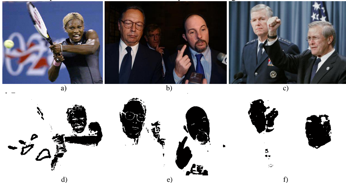
Fig. 2. Example of segmentation of color images from FDDB base on pixels of “skin” and “non skin”: a – b) original color images; d – f) binary masks, received during the usage of model of skin color
