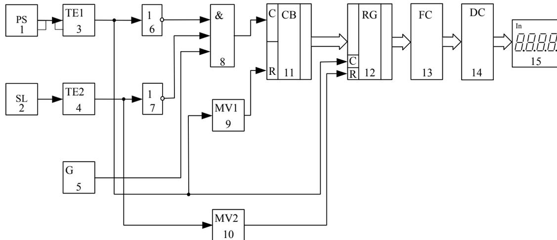
Fig. 4. Structure of the device for diagnosis of drum-block brake the tram-car
