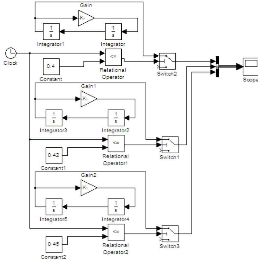
Fig. 2. Computer model, intended for diagnostics of drum-block brake
