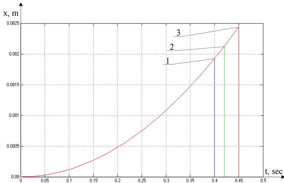
Fig. 3. Graph of brake spring drive elongation while operation: 1)  $t_1=0,4\text{sec}$ , 2)  $t_1=0,42\text{sec}$ , 3)  $t_1=0,45\text{sec}$
