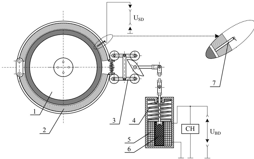
Fig. 1. Construction of drum-block brake of electric-driven tram-car: 1 – brake drum, 2 – brake lining, 3 – mechanism of brake drive, 4 – brake spring, 5 – coil of brake solenoid, 6 – drive of solenoid core, 7 – rod, made of light-weight alloy (diameter 3-6 mm)
