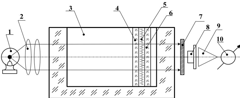
Fig. 2. Structure scheme of the device for the research of gas humidity analyzer characteristics
