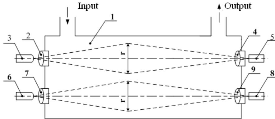
Fig. 1. Optical scheme for two-channel gas humidity analyzer
