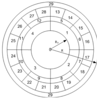
Fig. 2. Segmentation scheme of the spotted image of laser beam
