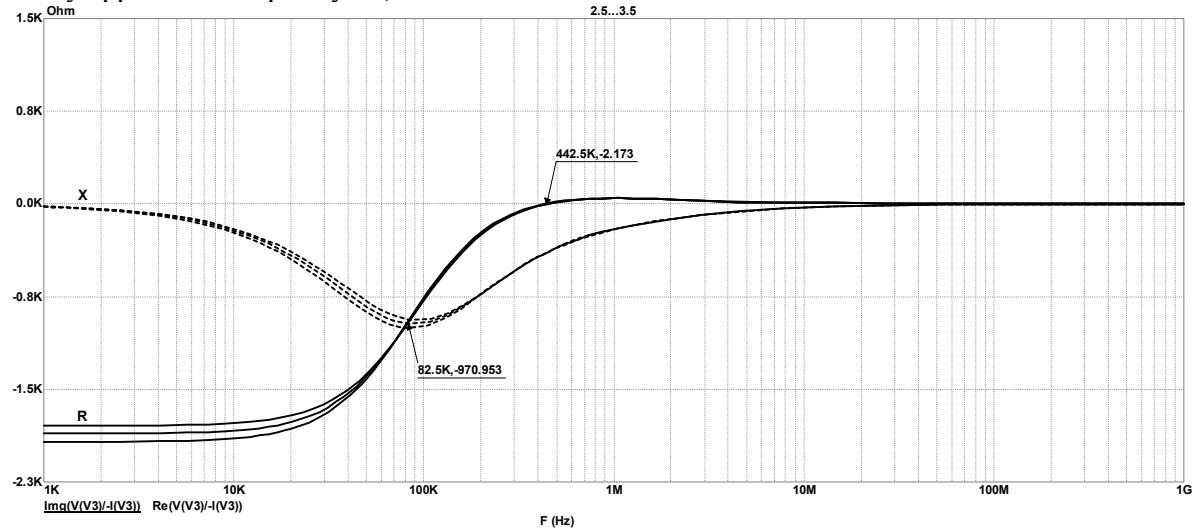
Fig. 4. Frequency dependence of active and reactive components of full resistance of active component BMD on BTSNR
