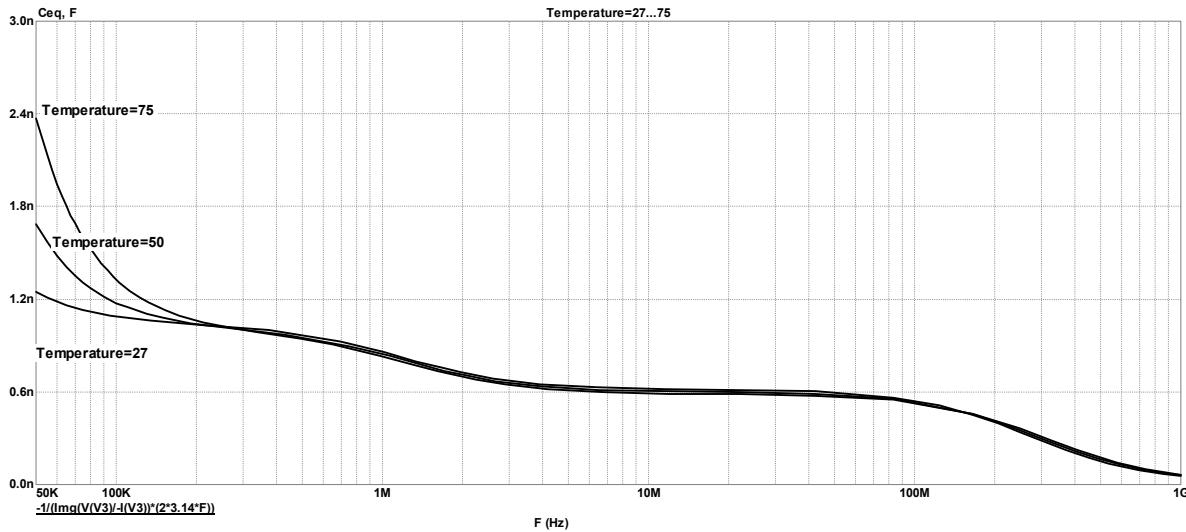
Fig. 8. Dependence of change of equivalent capacity of active component of BMD on BTSNR on frequency with 27, 50, 75 °C
