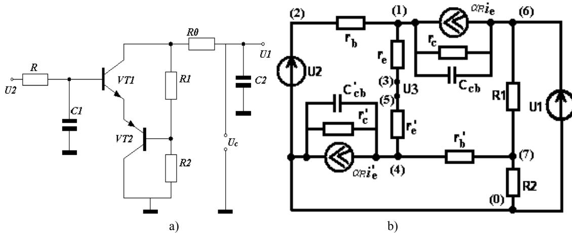
Fig. 1. Electric circuit (a) and equivalent circuit (b) of active component of RMD on BTSNR
