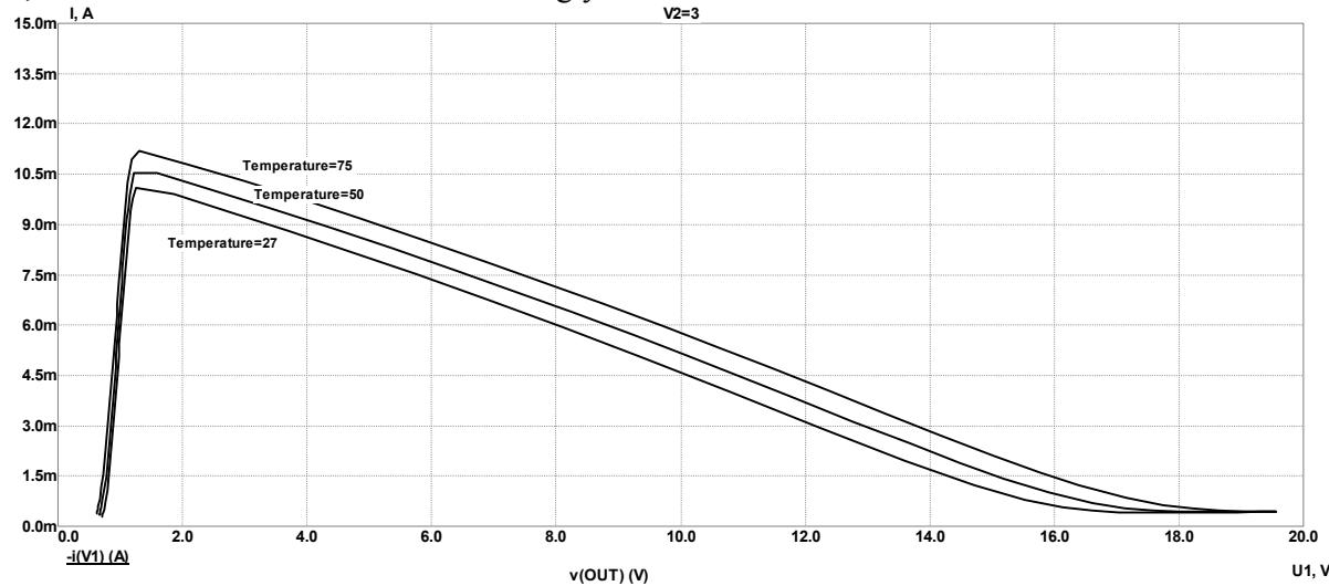
Fig. 7. CVC of active component of BMD on BTSNR under different operating temperatures with controlling voltage of 3 V
