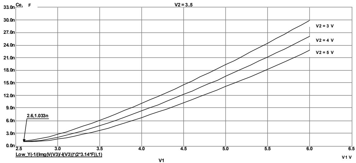
Fig. 6. Dependence of equivalent capacity change of active component BMD on BTSNR on voltage supply with different controlling voltage 3...5 V
