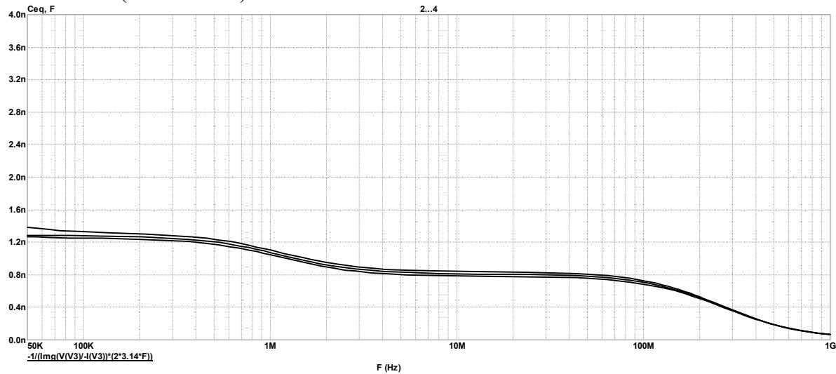
Fig. 5. Dependence of equivalent capacity change of active component BMD on BTSNR on frequency
