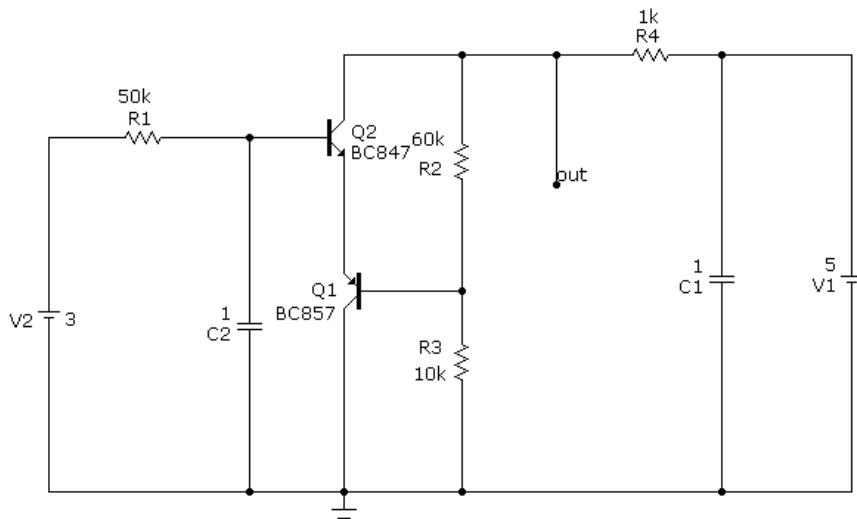
Fig. 2. Electric circuit of active component of BMD on BTSNR in the environment of MicroCAP
