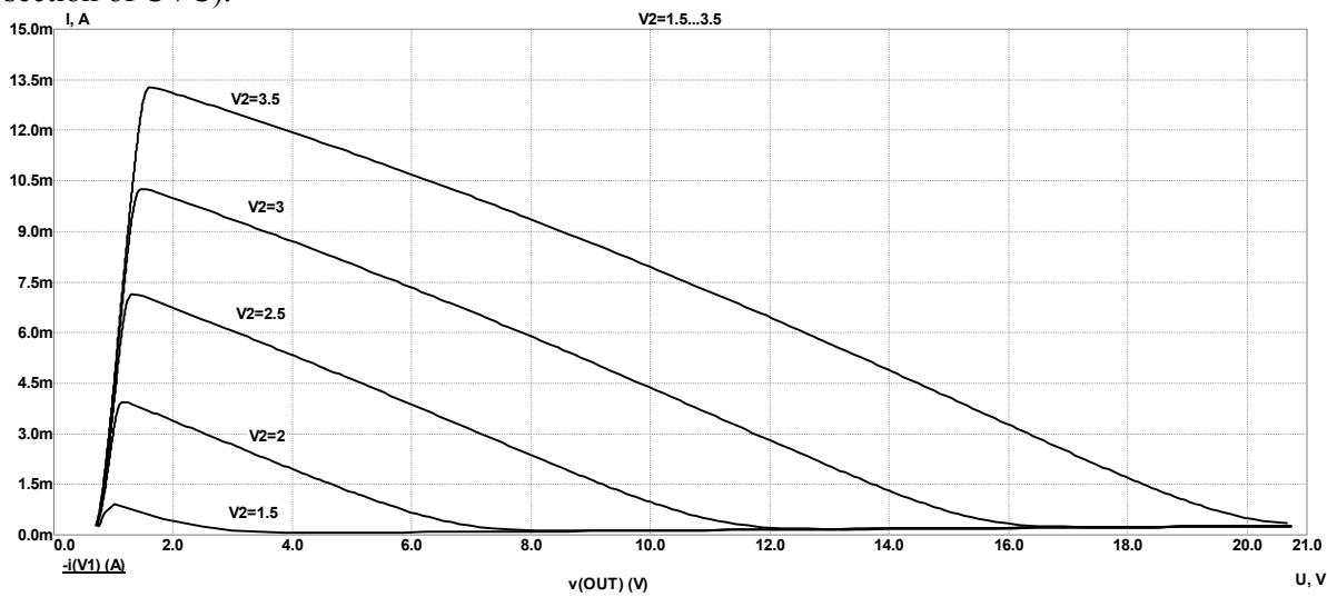
Fig. 3. Current-voltage characteristics of the researched equivalent of capacity on bipolar transistor structure with negative resistance
