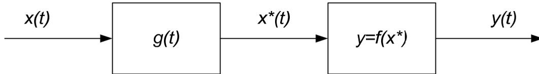
Fig. 2. Structure of dynamic object with allocation of time-lagging linear part and lag-free non-linear part
