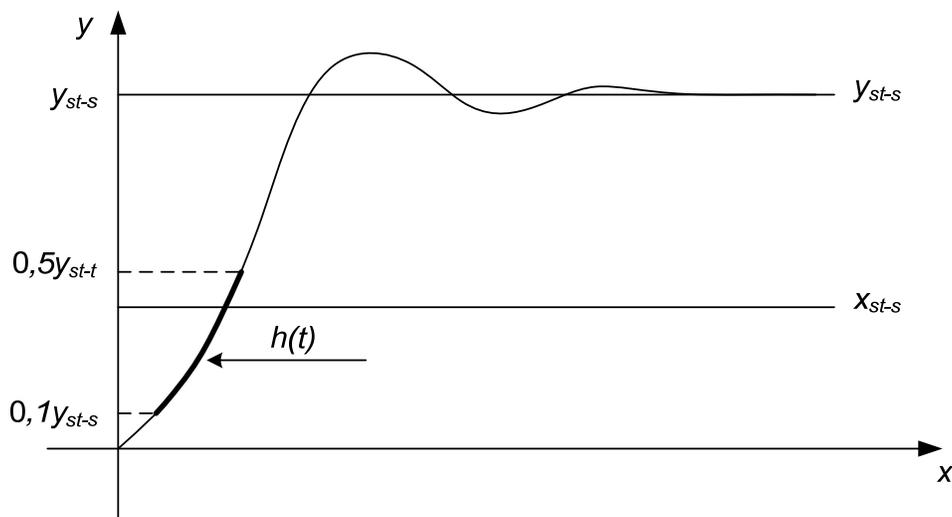
Fig. 3. Diagram of transitional process in the dynamic object after submitting the staged influence on the level of its steady-state value to the input
